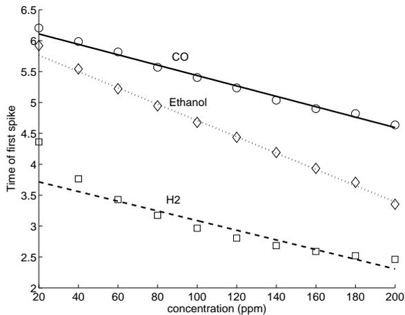
Fig. 10. Absolute time of the first spike of the generated spike train versus gas concentration, for ethanol, carbon monoxide and hydrogen.
