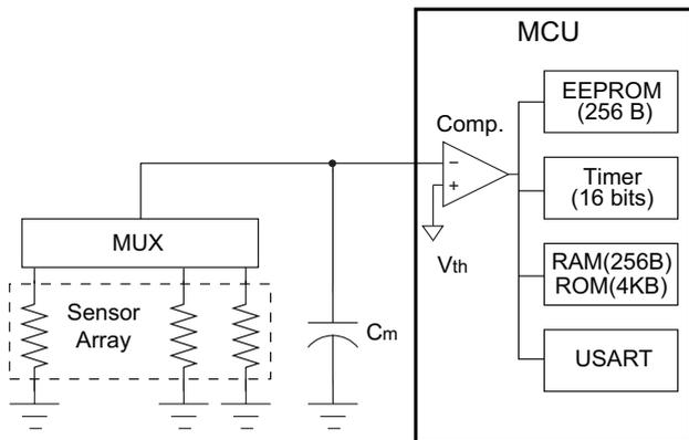
Fig. 2. Diagram of the resistance-to-time readout circuit. It utilizes the MCU comparator, with only one extra capacitor and one analog MUX added into the system. Note that the internal reference from the MCU is used to generate  $V_{th}$  to fully utilize the MCU available resources.
