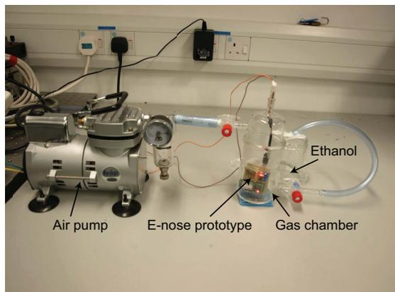
Fig. 8. Portable demo prototype. The compact E-nose system is placed inside a gas chamber. An air pump is connected to the gas chamber in order to provide a stable sensing environment for the system. Gas sensor resistances are first digitized then are transmitted to PC/PDA wirelessly using the Bluetooth module.
