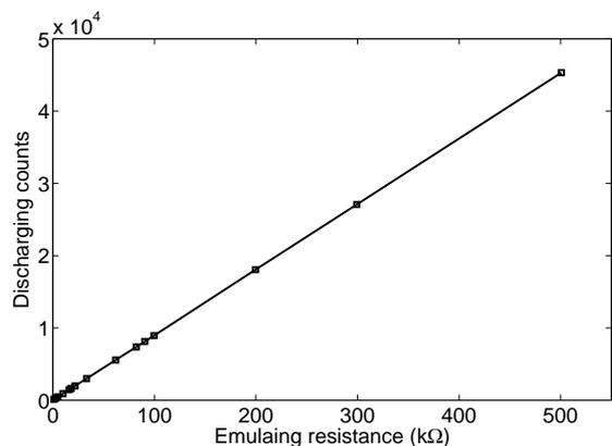
Fig. 7. Measured discharging count using different resistances for the readout circuit characterization.
