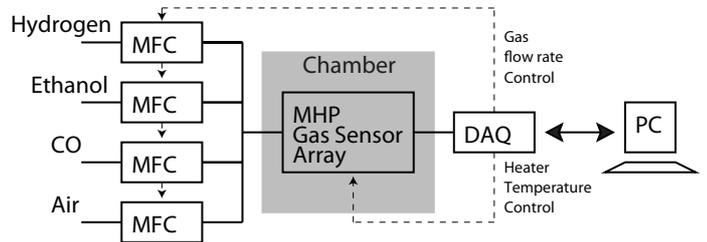
Fig. 4. Experimental setup used to characterize the sensor array.
