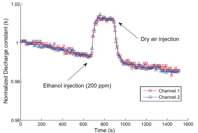
Fig. 6. Typical relationship between the normalized discharge constant  $k$  and two multiplexed channels when the two standard resistors are exposed to ethanol.
