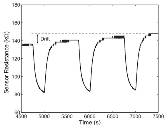
Fig. 5. Typical sensor response to ethanol. The sensor was initially exposed to air then exposed to ethanol for 3 times. It is exposed to air for sensor resistance recovery. Note that the sensor resistance is not able to fully recover to the original value due to drift.
