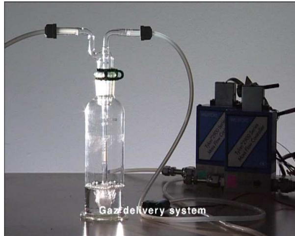
Figure 3: **Olfactometer.** The gas delivery system for *calibration method 1* consists of two micro-pumps (Diaphragm pumps from Sercom 2002 0.35 l/min), two airflow controllers (Tylan mass flow controllers 2900), one bubbler and a data acquisition system (the robot).
